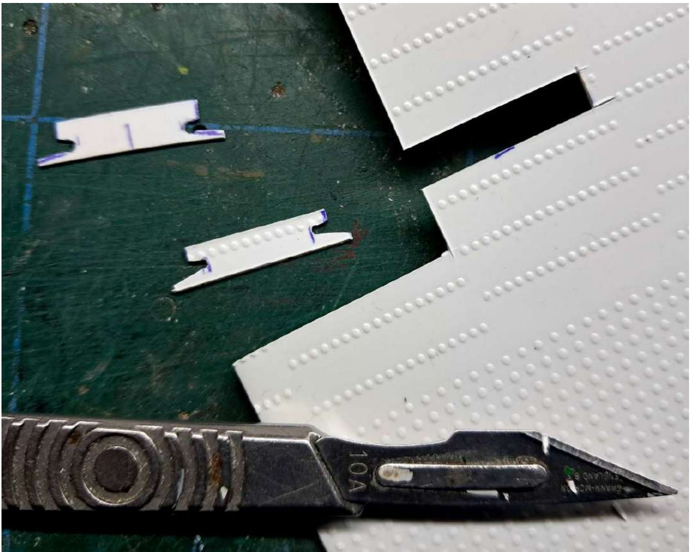
Cutting the tank support from plasticard with moulded rivets (origin uncertain!)
