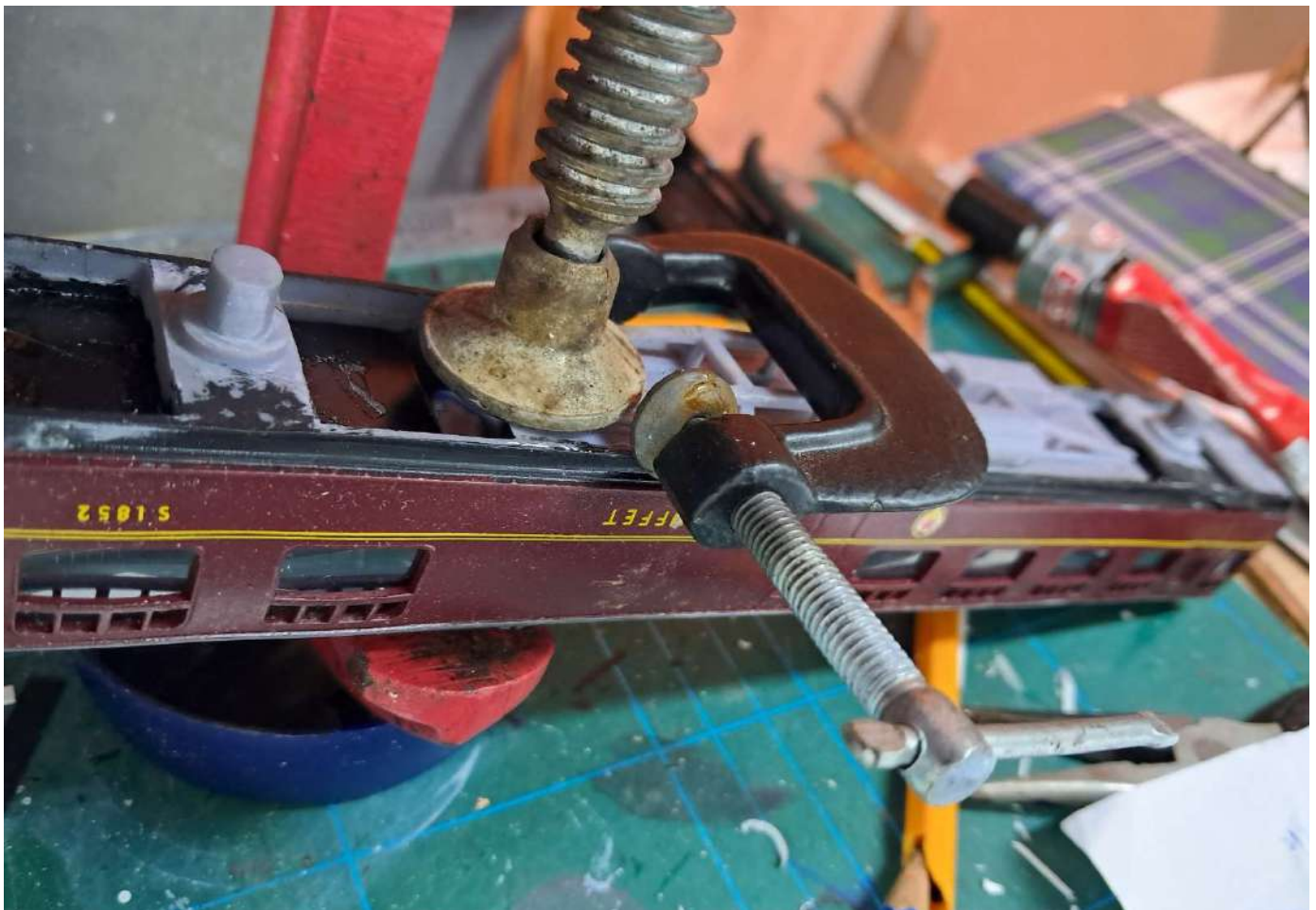
Assembly of the buffet car, with an attempt to correct the distortions.
